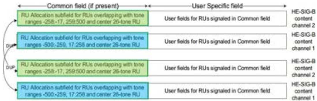
Figure 27-30—HE-SIG-B content channels and their duplication in an 80 MHz PPDU
