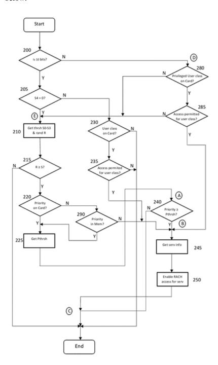
33. The judge explained the disclosure as follows. The first decision diamond 200 asks whether the 10- or 13-bit process should be followed. If there are 13 bits, the system proceeds to diamond 280. At this point, the system carries out two checks: first, is a user class stored on the mobile's access authorisation card (i.e. on its SIM card); secondly, if so, is that user class "normally privileged" or "privileged"? This is described in the specification as follows:
